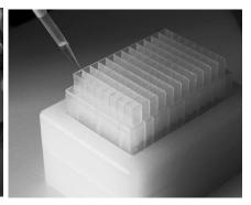
Place the plate over a collection vessel and recover the glycans by eluting with 4 x 0.2 mL of Wash B.
