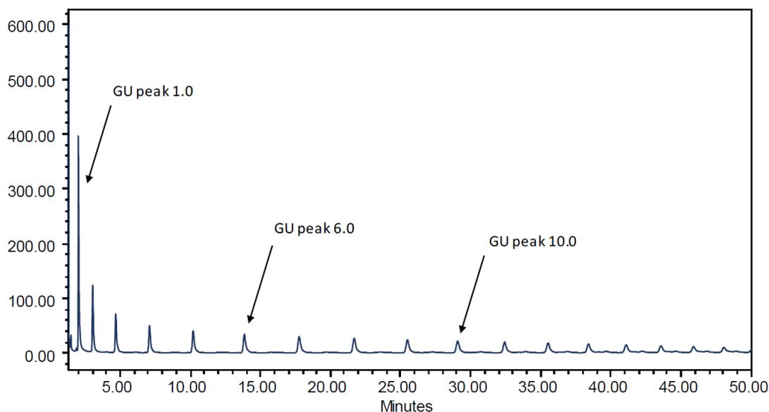
Figure 1: typical fluorescence trace of CPROC-GHP-30
