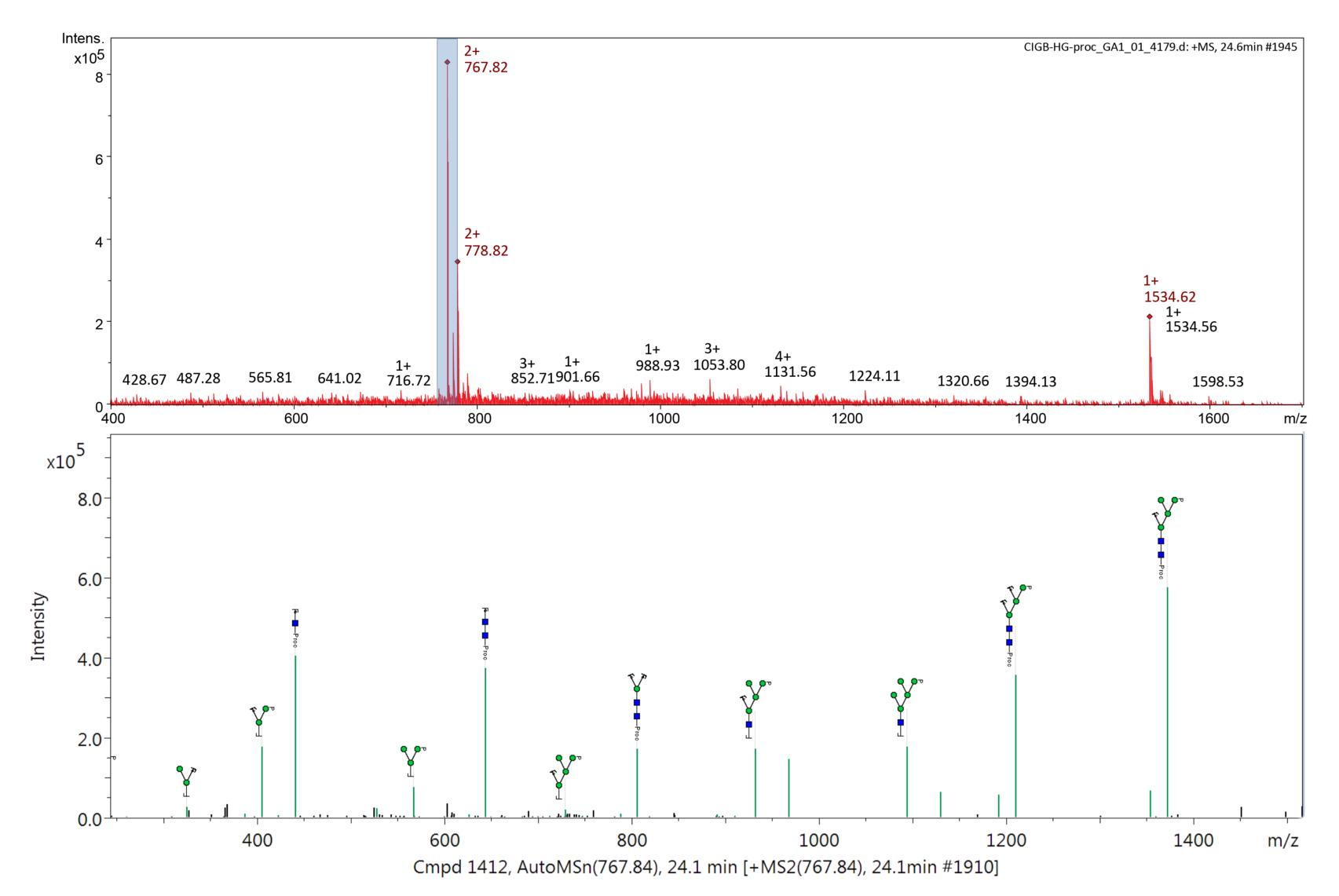
Figure 2: MS and an MS/MS of glycan mass 767.82 m/z using the Bruker amaZon Speed ETD – good fragmentation characteristics but mass accuracy not sufficient to determine whether the glycan was sulphated (767.7874 m/z) or phosphorylated (767.7922 m/z)
