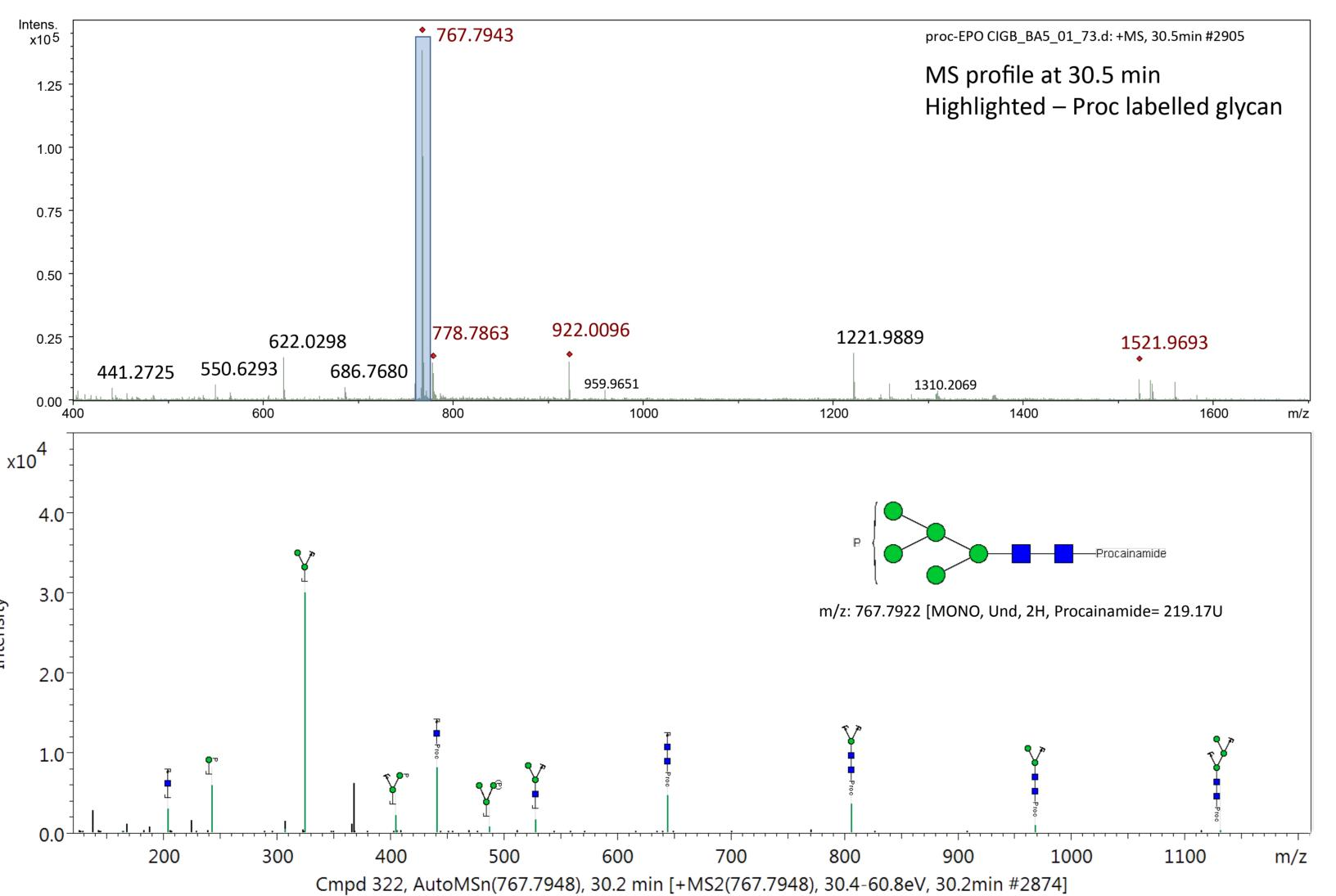
Figure 3: MS and an MS/MS of glycan mass 767.7943 m/z using the Bruker impact II QTOF – this instrument, designed for sub 1ppm mass accuracy identified the glycan to have the mass corresponding to a MAN5 glycan with a single phosphorylation. The glycan was identified using our EPO database in the Bruker ProteinScape 4.0 software.
