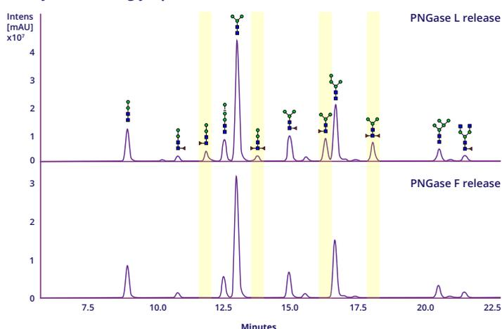
**Figure 1.** HILIC-UHPLC stack plot analysis of procainamide labelled N-Glycan Release from Honey Bee venom glycoprotein released with PNGase L (LZ-PNGase L-50); (top) and corresponding sample digested with PNGase F (LZ-rPNGaseF-kit) (bottom). Peaks from top chromatogram are labelled with glycan structures.
