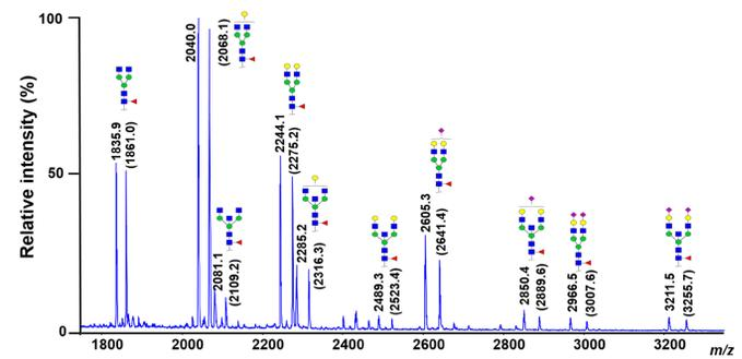
Fig-1: MALDI-TOF-MS spectrum of the <sup>12</sup>C and <sup>13</sup>C permethylated human-IgG N-glycan standards from Ludger (Cat# Cpm13C-IgG-01 and Cpm12C-IgG-01). <sup>13</sup>C was spiked with <sup>12</sup>C on the same sample spot to show the comparison of relative quantities of the major IgG N-glycans. The mass values shown in the spectra are [M+Na]<sup>+</sup> of permethylated glycans, with <sup>13</sup>C permethylated masses in parentheses.
