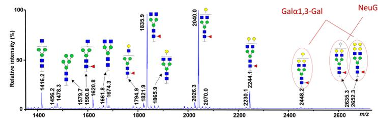
Fig-2: MALDI-TOF-MS spectrum of IgG1 mAb N-glycans permethylated on the liquid handling robot. Note: Galα1, 3-Gal epitope and N-glycolylneuraminic acid (NeuGC) are non-human glycosylation features, reflecting possible critical quality attributes (CQAs) due to the potential immunogenic characteristics of the mAb identified after permethylation.
