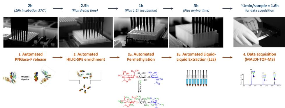
Scheme 2: LongBow system tuned for a largely automated and HT glycoprotein sample preparation workflow for (1) N-glycan release, (2) hydrophilic liquid interaction chromatography (HILIC)-solid phase extraction (SPE) of glycans, (3a) permethylation of released glycans, (3b)liquid- liquid extraction (LLE) and (4) Data acquisition.
